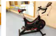
Ergometer for measuring maximal anaerobic power
